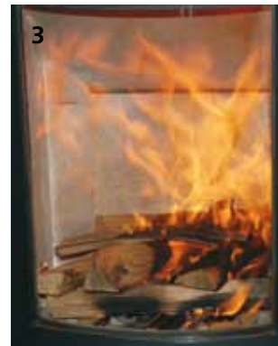
Make sure there is plenty of air so the flames are bright.
